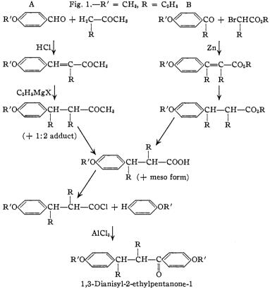
This has been accomplished as shown in the flow sheet in Fig. 1. The key compound is the racemic form of  $\alpha$ -ethyl- $\beta$ -anisylvaleric acid.
